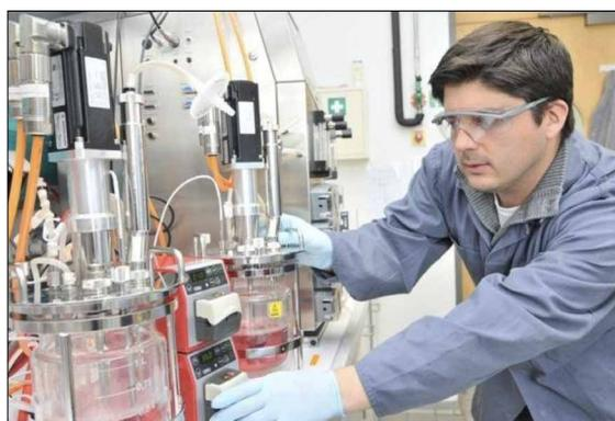
**Figure 4.** When the cells reach a high concentration, they are infected with virus, die off, and the virus is harvested. At that point, the process of growing a new batch of cells begins again. MPI-DCTS sought a way to continually harvest, and to do so, group member Felipe Tapia (shown here), added a secondary bioreactor designed solely to grow cells and feed the primary/infective bioreactor. (Photo courtesy of MPI-DCTS.)
