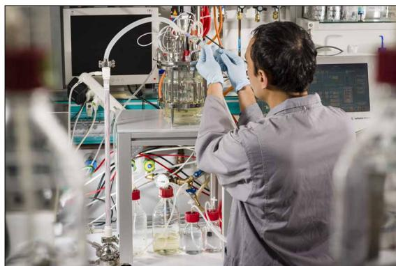
**Figure 3.** A main focus of MPI-DCTS researchers is figuring out how to support the increasingly higher numbers of suspension cells grown in a bioreactor [a 1-liter bioreactor connected to a hollow fiber membrane (left) and an ATF2 system is shown here]. This work involves developing a variety of perfusion systems to maintain nutrient-rich medium in the bioreactor, and remove used medium and waste the cells, without harming the fragile growing cells. (Photo courtesy of MPI-DCTS/Ehl.)
