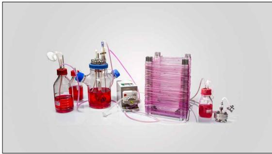
**Figure 5.** Advancing with the continuous-harvest approach, researchers redesigned the primary bioreactor from a single container to a thin 100-m-long tube. Cell-containing medium is sent into the tube one small volume, or “plug,” at a time. A bit of air separates the plugs, which are infected with virus individually. A spin-off company ContiVir is developing the continuous tubular bioreactor system further. (Photo copyright: www.contivir.com.)
